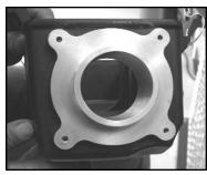
15. Install the provided adapter into the air box. Make sure the holes line up.
