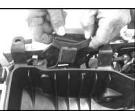
10. Remove the Engine Control Unit Assembly band.
