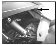
8. Remove the bolt that goes into the air box (left side).
