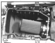
20. Install the K&N Filtercharger® onto the adapter. Securely tighten the clamp.
