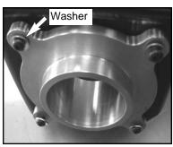
16. Install the four provided buttonhead bolts and four washers on the outside of the air box. Note: The washers will go in between the bolts and the adapter.
