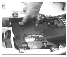
3. Unclip the four air box lid hooks.
